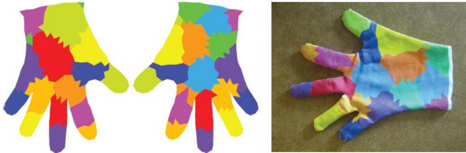
Figure 2.14: Glove design consisting of large colour patches accounts for camera limitations, self-occlusion, and algorithm performance. The length of glove is 24cm
