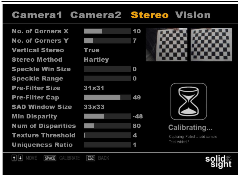
Figure 4.11: Interface for Stereo Calibration and Configuration of the Disparity Map
