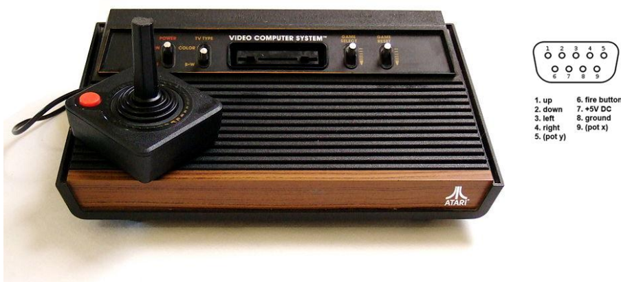
Figure 1.15: Atari 2600 four-switch "wood veneer" version, dating from 1980-1982 with CX40 joystick and Computer port view of the Atari standard connector (insert right)
