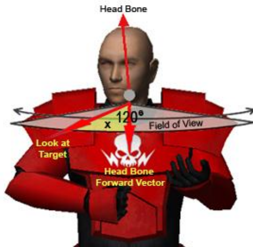
Figure 4.8: Field of View & Shortest Arc Algorithm for calculating Look-At Inverse Kinematics
