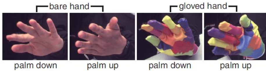
Figure 2.15: The palm down and palm up poses map to similar images for a bare hand. These same poses map to very different images for a gloved hand
