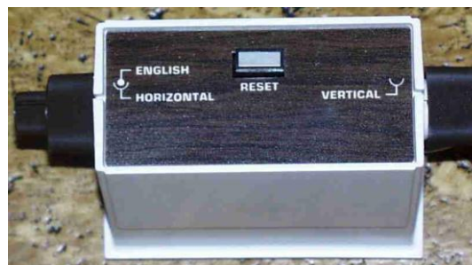
Figure 1.13: Magnavox Odyssey's potentiometer joystick
