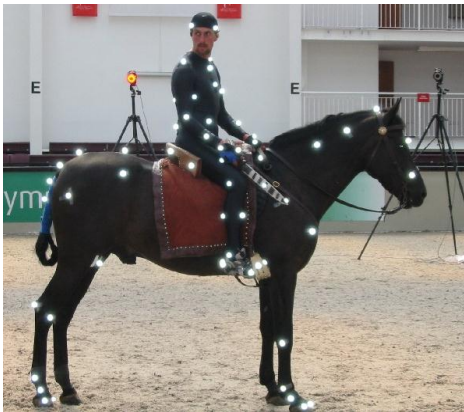
Figure 2.1: Actor and Horse wearing markers as part of MotionAnalysis's Passive Optical Motion Capture System
