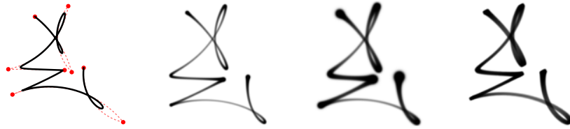
Figure 1: Sigma Lognormal trajectory, the corresponding action plan (in red) and renderings with different kinematic dependent brushes.
