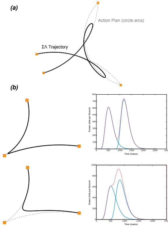
**Figure 3:**  $\Sigma\Lambda$  Model. (a) The action plan that defines a complex trajectory. (b) Smoothing trajectories by varying the time overlap of the stroke velocity profiles (dashed red: the trajectory velocity profile. Turquoise: the single stroke velocity profiles).
