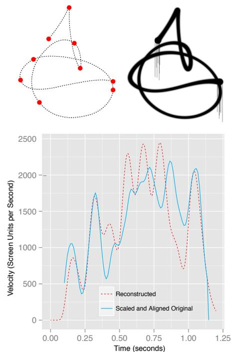
**Figure 12:** Fitting a  $\Gamma\Lambda^*$  trajectory. Top Left: the input contour and corresponding segmentation points. Top Right: the generated trajectory. Bottom: The velocity of the generated trajectory (red) overlapped with a manually scaled and aligned version of the input velocity signal (turquoise).
