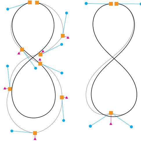
**Figure 4:** A comparison between  $\Sigma\Lambda^*$  (left) and  $\Gamma\Lambda^*$  (right) models in the task of describing a “figure 8”. In orange (■): the virtual target positions. In turquoise (●): the handles used for manipulating the  $\phi_j$  parameters (left) or the  $\phi_{1j}$  and  $\phi_{2j}$  parameters (right). In green (▲): the handles used for adjusting the  $\Delta t_j$  parameters.
