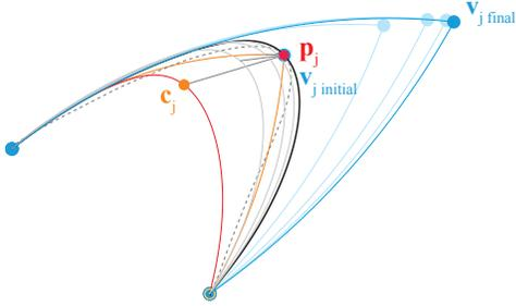
**Figure 10:** Iterative fitting: The initial action plan (orange) generates a trajectory (red) that is scaled with respect to the original (dashed grey). Through successive iterations the initial virtual target position moves until the corresponding point along the trajectory (orange circle) converges towards the input segmentation point (red circle).
