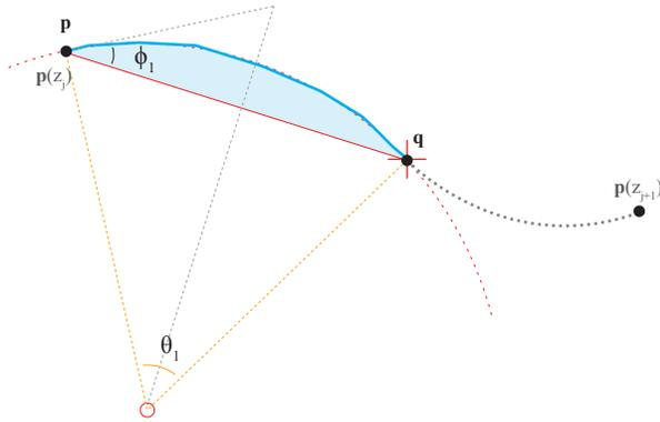
**Figure 8:** Computing  $\phi_1$  by fitting a circular arc between the first point of the contour section  $\mathbf{p}(z_j)$  and the inflection at  $\mathbf{q}$ .  $\phi_2$  will be computed similarly between the inflection (red cross) and  $\mathbf{p}(z_{j+1})$ .
