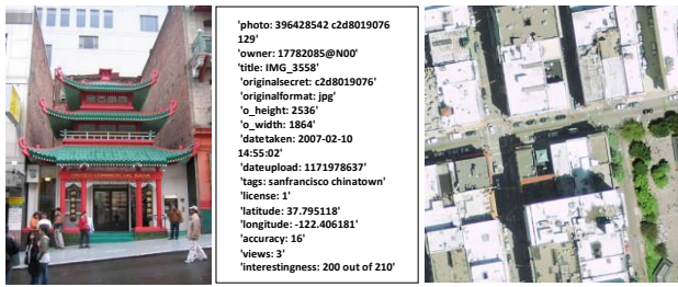
Figure 1 - Example of metadata extraction from ground level image (image, left) to obtain geo-tag, text descriptions etc (text box, center). The geo-tag is next used to find aerial imagery around the geo-location and finally a suitably sized aerial image patch is extracted around that location to provide aerial data (image, right).
