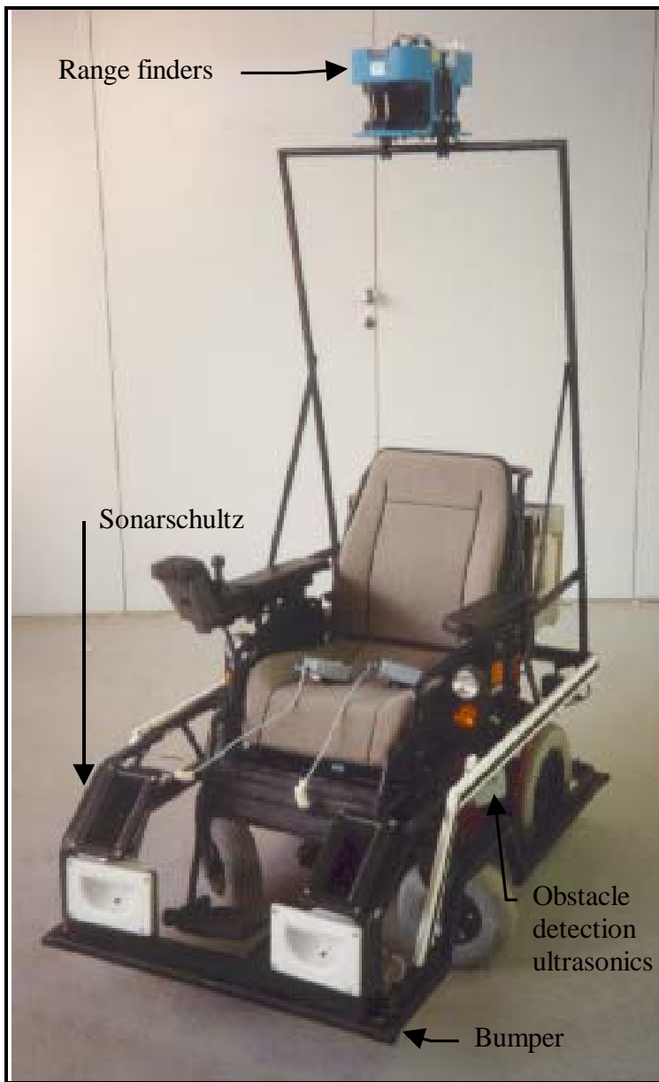
Figure 8 - Wheelchair with the Positioning sub-system installed.
