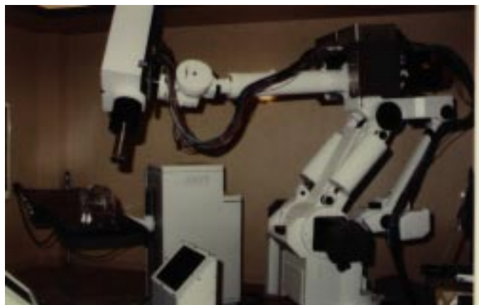
Fig. 1. Robotic radiosurgical system, patient table, phantom skull, x-ray cameras
