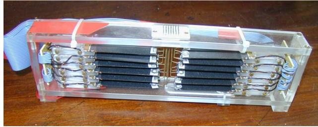
**Fig. 4** Single-digit stimulator with 25 contactors over  $1\text{ cm}^2$  on the fingertip.
